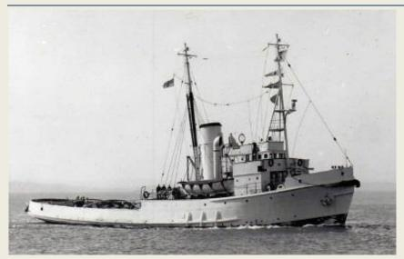
Allocated to SNO Selsey to tow Phoenix and Whale units. Built by Cochrane & Sons Ltd., Selby. Assurance tug. L156'6. B35'. D16'6". 630grt. 1350ihp 3cyl TE oil fired engine by C Holmes Ltd., Bunkers 250 tons. BP13.5T. 24-3-1943 Launched for UK Admiralty, named Ant. 26-6-1943 Delivered UK Admiralty, re- named Antic 1943. Loaned
