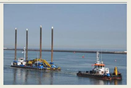
Her grt is 100 tonnes and dwt 133 tonnes. The two Caterpillar main engines develops a total output of 1,268 kW (1,722 hp). She has a speed of 9 knots and is classed Bureau Veritas *(Photo: Joop Marechal)*
