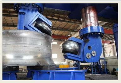
Damen Marine Components will supply a total eight 5,050 millimetre propeller nozzles for four ultra-long distance towing and anchor handling vessel newbuildings. They are the largest nozzles that DMC will have manufactured with its spinning machine technique to date. The order was granted by Caterpillar Propulsion of Gothenburg. Caterpillar is to provide the complete main propulsion units and has commissioned Damen Marine Components, a member of the
