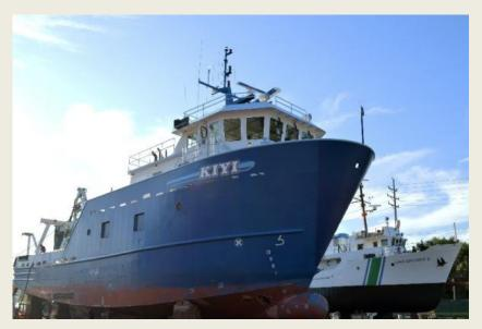
The research vessel was hauled out using the 770-ton capacity Marine Travelift at Great Lakes Shipyard. The repair contract that started on September 5, 2014 includes: Drydocking; Routine Repairs and Maintenance; ABS Five-Year Survey and Inspection for Load Line; Clean & Paint Underwater Hull, Decks & Superstructure; Overhaul Main Engines & Generators; Maintenance of Propulsion & Steering Systems; Modify
