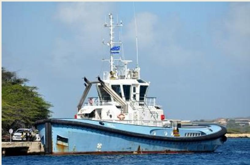
was introduced to the market during the ITS Conference held in Hamburg in 2014. The tug has been built with the following specifications: Length o.a.:30,30 m; Breadth o.a.:13,40 m; Draft:4,75 m; Max Speed:13,5 Kn; Bollard Pull:65 tons. Class : BV I +HULL · MACH ESCORT TUG, AUT UMS, Unrestricted Navigation. *(Photo: Kees Bustraan)*
