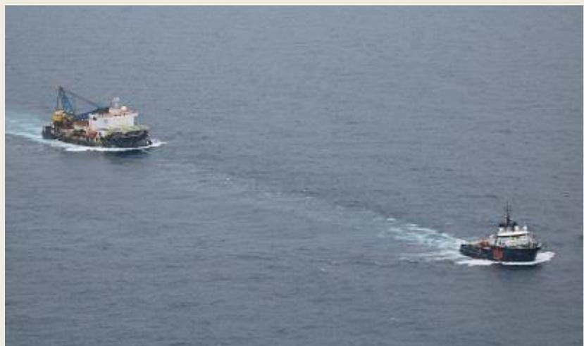
+ 100 A5 E2 Deep Sea Tug Boat (Nav-A4) + MC E2 AUT, FF1, DP2. She has a Length o.a. of 65,00 m; Length b.p. of 59,06 m; Beam o.a. of 18,50 m; Depth to maindeck of 8,50 m; Max. draught of 7,50 m; Gross tonnage of 2.789 mt and a Deadweight of 2.817mt. She has a Bollard pull of 219 mt cont. / 232 mt max a Maximum free sailing speed 16,0 knots with a Service speed 10,5 knots. *(Photo: Capt. Lawrence Dalli - www.maltashipphotos.com)*
