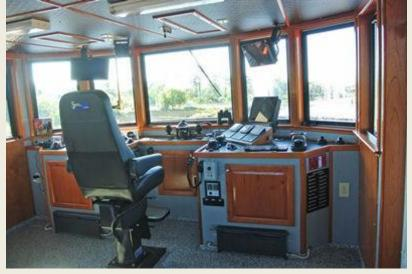
gallons of fuel, 8,000 gallons of water, 500 gallons of lube oil, 1,000 gallons of waste oil, and 1,000 gallons for zero discharge provisions. An extensive set of wheelhouse electronics includes two Halo 4-pulse compression radars, 16-inch touch-screen chart display, satellite compass, AIS, autopilot, depth sounder, and weather station all manufactured by SIMRAD. There are also three radiophones, a sat phone, and a bridge monitoring system. Electrical power is provided by two Cummins QSB7-
