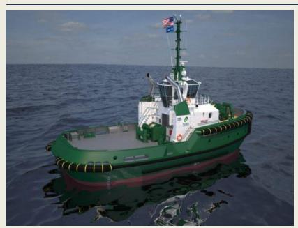
US-based Foss Maritime and Netherlands-based Damen Shipyards have signed Memorandum of Understanding the construction of at least ten next-generation ship assist and escort tugs for the US market. The first four in the series will be constructed at the Foss Shipyard in Rainier, Oregon, with delivery planned for 2019. The tugs will be built to Damen ASD 2813 design, which has been modified to meet the demands US tug assist
