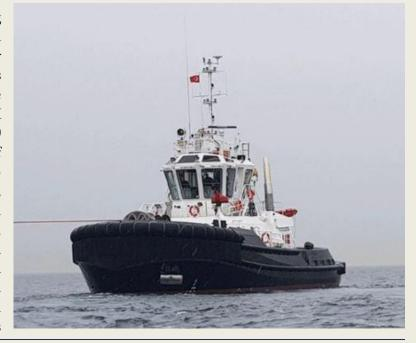
for Italy will be built to RINA class and Italian flag requirements and will be powered by pairs of 1500kW Caterpillar engines. These turn Schottel azimuthing Rudderpropellers to give a minimum of 50 tonnes bollard pull. The vessels will be delivered by the end of 2017. (Sanmar)
