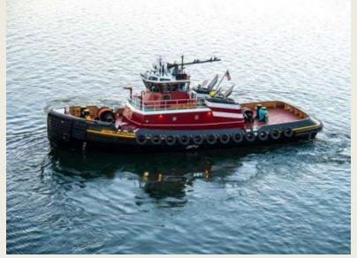
JonRie Intertech, has supplied its sixth ship set full 90 ton line pull winch for installation on McAllister Towing & Transportation Company, Inc.'s 5,150 HP twin Zdrive reverse tractor tug Jeffrey McAllister. Built by Eastern Shipbuilding, Panama City, FL, the 92' (30 meter) x 36' (11 meter) tug has a bollard pull of 75 tons and is the latest addition to the McAllister The JonRie Series 250 Escort Winch was Fleet. designed to handle in the recover mode the full bollard pull of the
