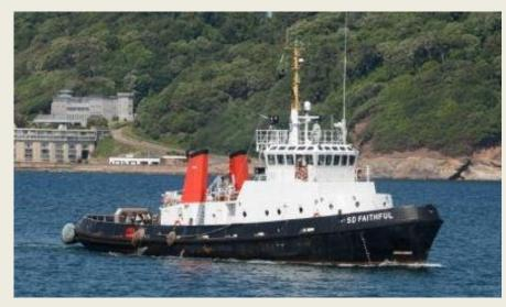
Serco Marine Services has returned its tractor tug SD Faithful to service for the UK Royal Navy after a major overhaul. The twin tractor tug's engines and generators were updated reconditioned and by Royston at A&P dockyard in Falmouth, UK, so it could return to push-pull ship handling operations in Devonport. Royston said the work involved
