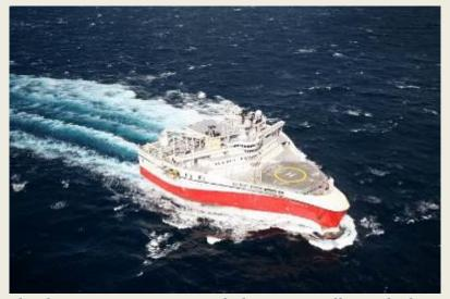
certainly have attracted attention by her unusual shape -the bows and front end of a huge ship, but very little or nothing behind the bridge. The Norwegian vessel is the second in the ultra-high capacity Titan class, with a deadweight of 7000 tons and a length of just 104 metres but 70 metres in the width. The reason for this oddity is to facilitate the streamers that the vessel tows behind her at sea and which are used in the seismic signalling.
