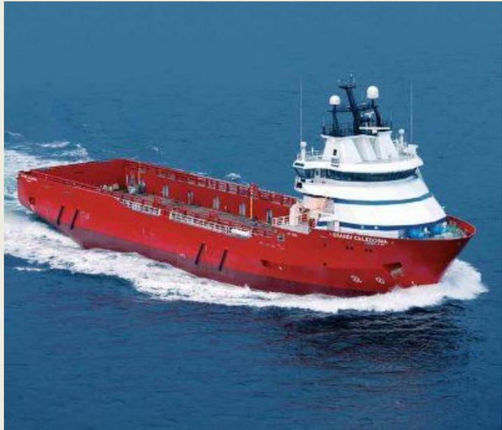
designed for field installation operations across a wide range of water depths and environmental conditions. **Skandi Skansen** is also classified as a CSV as the vessel is also equipped to carry out construction support activities. The 2003-built **Skandi Caledonia** is of an MT 6000 design. It is used to transport materials, supplies and personnel to and from offshore drilling rigs and platforms. *(Source: offshore Energy Today)*
