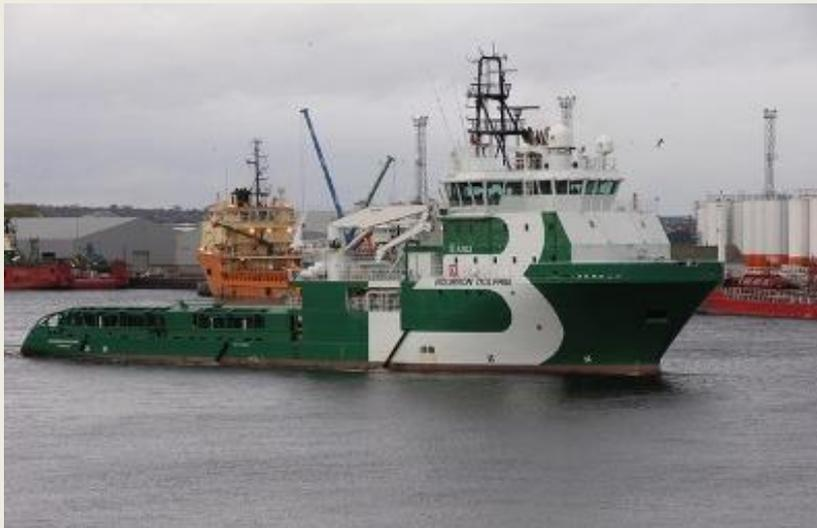
The Ulstein A102 **Bourbon Dolphin** entered service in late 2006 and capsized with the loss of eight lives while anchor-handling at the **Transocean Rather** in April 2007. This then might be the only claim to fame for the vessel type, of which no more have been constructed. It appears that the intent of the design was to produce a high specification vessel in a smaller hull than the Ulstein A101, and here I might have to declare a
