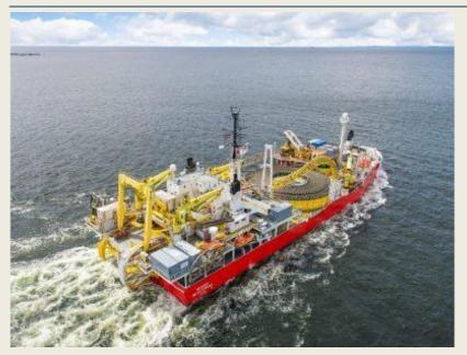
Installation of a subsea power between Norway cable Germany has started. The first metres have been laid on the seabed in Vollesfjord in Vest-Agder. Once completed, the new cable, NordLink, will be one of the world's longest power cables, and will provide the first direct link between the Norwegian and German power grids. The entire interconnector is 623 kilometres in length, and 516 kilometres will be installed as a subsea cable. "The first part of the cable will be installed this summer.
