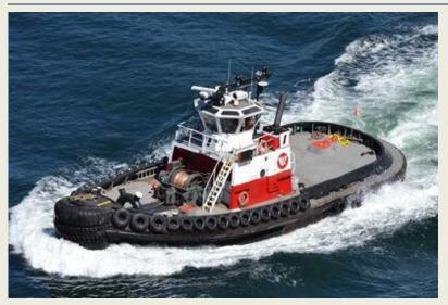
Cates tug **Cates 1** (Imo 8703218) was seen outbound in Vancouver harbour bound for Sechelt B.C. on the Sunshine Coast of B.C. on July 29, 2017. The tug is one of a Robert Allen design. The Cates Zdrive class tugs are characterized by their light displacement, simple and cost-effective outfitting and construction, and "slippery" hull form, ideal for fast manoeuvring, fast side-slip, and rapid response. She was built in 1986 by West Coast Manly
