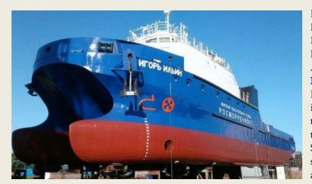
**SDS18** built for Project Marine Rescue Service of Rosmorrechflot (Federal Marine and River Transport Agency) and named Igor Ilyin, the shipyard told IAA PortNews. Okskaya Shipyard is the first company in Russia to start building vessels of this type. The ship of Project SDS18 is intended for support of diving operations at depth of up to 60 meters
