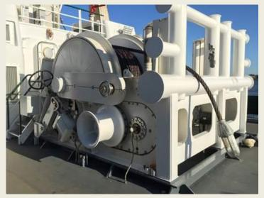
For several decades, Rapp Marine has designed and delivered towing winches for workboat market. Combining the best ideas from Rapp's past work in the other commercial industries and recommendations from the tugboat operators, Rapp Marine has developed long lasting and dependable towing winches. These past towing winches have mainly been powered using hydraulic systems in the North American market. Rapp Marine has previously delivered electric winches to commercial vessels in other industries
