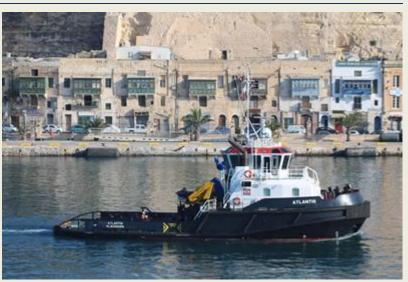
mtrs. The MTU diesel engines develops a total output of 3,680 kW (5,000 hp) with a free sailing speed of 12.5 knots. She has a grt of 365 tons and a dwt of 109 tons and is classed Bureau Veritas. *(Photo: Capt. Lawrence Dalli - www.maltashipphotos.com)*
