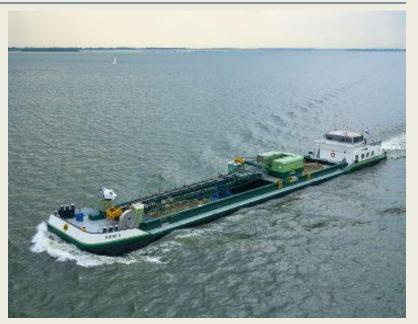
be used for dredging and rock dumping, Van den Herik said in its announcement. The **Prins 6** has an electric PLM 1217E crane of PLM Cranes. The crane regenerates energy when lowering the load, which perfectly suits within the hybrid character of the vessel. (*Source: Dredging Today*)
