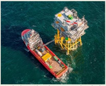
platform supply vessel that was equipped with a special Ampelmann gangway and was therefore suitable for the crossover manoeuvres, was used at the Gemini wind park during the project. The vessel operated by Vroon Offshore Services provided work and residential space for the project team consisting of 40 people as well as 20 crew members. This eliminated the need to transport the employees from the base port of Eemshaven and back every day. 934 trips were completed overall
