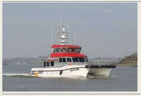
Workcats Blyth new multirole 17m work boat has successfully now completed its initial seatrials. The 'highbridge' vessel has been designed for both crew transfer complete with a wind turbine docking unit, and also hydrographic survey with an internal multibeam deployment carriage and an A frame on the transom. The helm position above the
