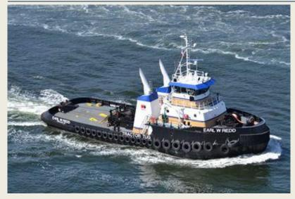
The Harley Marine Services 2017 built tug Earl W. Redd was seen towing an oil barge inbound Vancouver Harbour on the 15th July 2017. Built at Diversified Marine of Portland, Oregon, the Earl W. Redd measures 120 feet by 35 feet, with a loaded draft of 19 feet 3 inches. The tug features twin Cat 3516 Tier 4 Final main engines that will each produce 2,675 horsepower at 1,600 rpm. Each of the engines is paired with а selective catalytic
