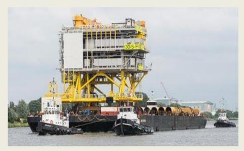
print of 36 x 36 meters, weighing 4,400 tonnes. Heerema Marine Contractors (HMC) is responsible for the execution of the transportation to the offshore location and will also perform the installation with HMC's SSCV Hermod in the Oseberg area in the Norwegian part of the North Sea, about 130 kilometers north-west
