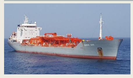
On 1 April 2017, the LPG Tanker "**Gemini Gas**" (GT 7,082 – DWT 9,490) experienced fire in the engine room about 132 miles south-east of Salalah, Oman. During the incident the vessel was on passage from Khorfakkan, UAE to Port Sudan, laden with 4.400 tonnes of LPG mixed. The vessel sustained severe damages due to fire and
