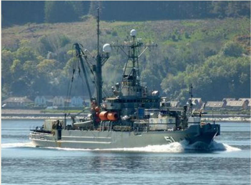
Draft of 17' (max.). Her free sailing speed is 14 knots. The four Caterpillar 399 diesel engines develops a total output of 4,200 hp on two shafts. *(Photo: Tommy Bryceland SCOTLAND)*
