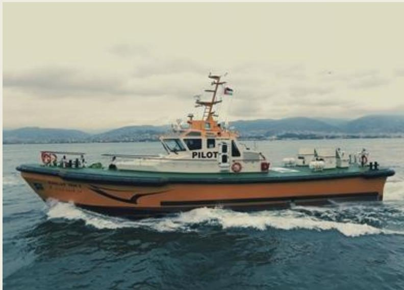
Macduff Ship Design is pleased to announce the successful trials and delivery of two 27m Pilot Vessels, **Marcap Tam 2**, built by Tor Marine in Turkey for Saudi Arabian owners. The vessel deliveries emphasise the continuing strong relationship between Macduff Ship Design and Tor Marine. At 26.70 metres length overall - a generous length for a pilot boat - 7 meters beam and 3.34 meters depth, the vessels are each designed to carry eight crew and four pilots and operate
