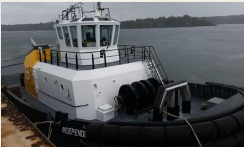
JonRie Marine Winches Commissions its new Container Master Series “220” Double Drum Escort Winch currently installed on the Tug **Independent** (new ASDs for Marine Towing of Tampa) The Container Master Series “220” Double Drum Bow Winch was designed for a larger capacity rope as can be seen from the photo. This concept used on the Panama
