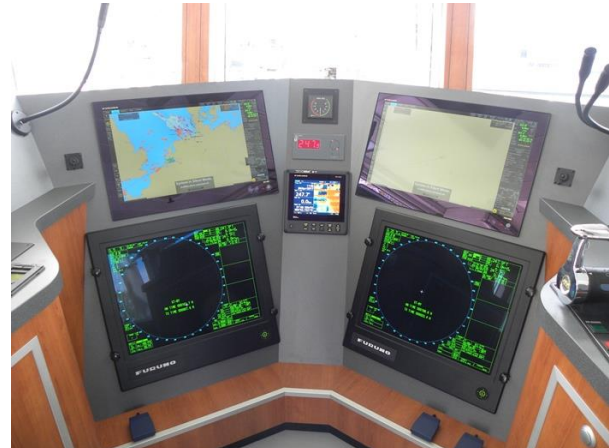
Radars forward bridge console view
