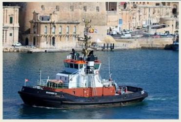
and 819 respectively. The tugs are owned by Bugsier Reederei und Bergungs AG – Hamburg; Germany. The **Bugsier 20** has a length of 30.55 mtrs a beam of 11,63 mtrs and a depth of 4.00 mtrs. The **Bugsier 21** has a length of 30.62 mtrs a beam of 11.65 mtrs and a depth of 4.00 mtrs. Both Voith Schneider propulsion tugs have the same two MWM-Deutz SBV9M628 diesel engines with an total output of 3,800 kW (5166 bhp). *(Picture Credit as Capt. Lawrence Dalli –*
