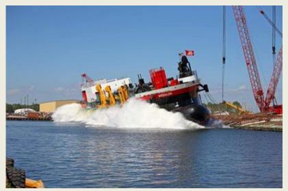
Eastern Shipbuilding is pleased to announce that on, Friday, March 31, 2017, it successfully launched the Trailing Suction Hopper Dredger, the M/V MAGDALEN. This 356' Twin Screw U.S. Flag Trailing Suction Hopper Dredger currently under construction at Eastern's Allanton Panama City, Florida facility. On a perfect sunny Florida day, the launch was hosted by Eastern's Founder and CEO Brian D'Isernia. Brian
