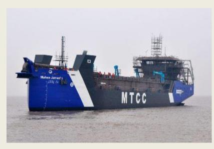
go-ahead. The dredger will be used for land reclamation, beach infrastructure and nourishment projects on several islands and resorts in Asia. TSHD Mahaa Jarraafu is equipped with the specially designed Easydredge dredging equipment, including the IHC dredge pump and a slender hull for increased speed and low fuel consumption. In addition, vessel has a 'world the dredging' equipment package, which includes an adjustable
