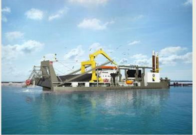
Merwede. It concerns a sister vessel of the 'Helios' which will be taken into service later this year. The new vessel will also have a total installed power of 23,700 kW, a pumping capacity of 15,600 kW and a maximum cutter capacity of 7,000 kW. The new cutters can dredge in extremely hard ground at depths ranging from 6 to 35 meters. The new vessel is expected to be
