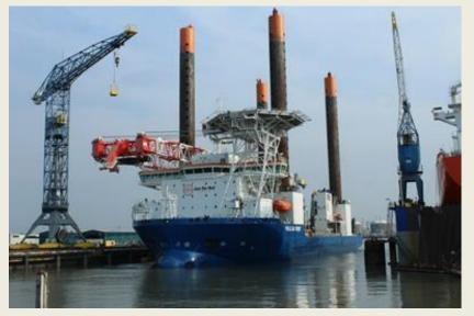
Jack-up vessel Vole au vent and TSHD Leiv Eiriksson. Damen Shiprepair & Conversion (DSC) has recently completed works in Vlissingen and Brest on two major vessels in the fleet of dredging and marine construction specialist Jan de Nul Group. One of these is the Vole au vent, a 140metre jack-up vessel built specifically for the installation of the latest generation of offshore wind turbines. The other is the trailing suction
