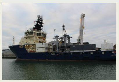
Danish engineering consultancy Geo and NCT Offshore have launched the drillship Freja as new strategic part collaboration. Freja is an S-Class ROV support DP2 vessel, and according to Geo is the only drillship of its calibre and type in the Nordic countries after the rebuild. The drilling setup aboard Freja is based on a system designed to provide optimised heave compensated drilling conditions. Department director
