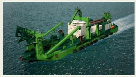
Royal IHC (IHC) has been awarded a contract for the design, construction and delivery of the 44,180kW self-propelled suction dredger (CSD) Spartacus, for DEME in Belgium. The newly built CSD will be 164 metres long. The concept and basic design for this mega cutter was done in close
