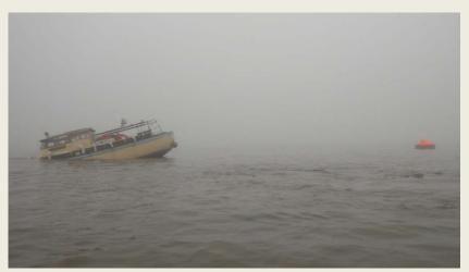
The UK Marine Accident Investigation Branch (MAIB) has released its report into the collision of the WWII-era training boat **Peggotty** and the ro/ro **Petunia Seaways**, and has concluded that the **Peggotty**'s use of an iPad as primary means of navigation was a key factor behind the accident.
