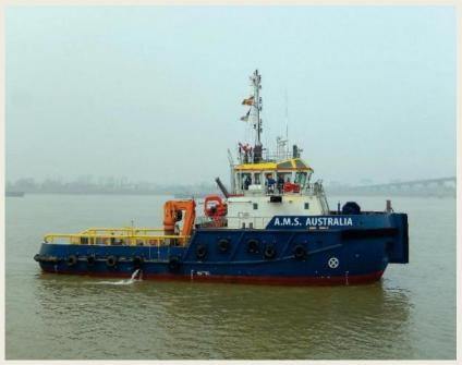
Australia Marine Services PTY LTD, a provider of quality tugs, workboats and barges in Australia and S.E. Asia. recently launched their 34-2,400kW metre anchor handling tug/offshore support vessel A.M.S. Australia in Shanghai. Powered by a pair of Cummins KTA50-M2 main engines, the tug achieved a top speed of 13.6 knots on trials and was certified with a bollard pull of 41 tonnes. For towing and anchor handling operations the tug is equipped with a hydraulic waterfall
