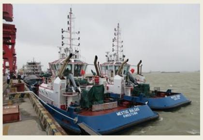
service speed of 11.5 knots. The accommodation is provided for ten crew. The boats have capacity for 110 m3 of fuel oil and 25 m3 of fresh water. Both vessels are outfitted with class-1 firefighting equipment. Mextug Lerma and Mextug Balsas have been delivered from Nantong, China to Lazaro Cardenas, Mexico by the Ship Delivery department of TOS (Transport & Offshore Services) from the Netherlands. Together with Azistern3360 tug 'Ranquel'
