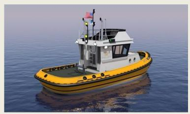
specifically for shipyard work, robust enough to endure long hours each day while minimizing the resources needed to operate and maintain it. The resulting tug is an attractive, compact, steel-hulled boat that can be operated by a single person. The 38' by 15' by 5.5' tug is currently under construction by San Diegobased boat-builders Marine Group Boat Works at its new solar-powered construction facility in National City,
