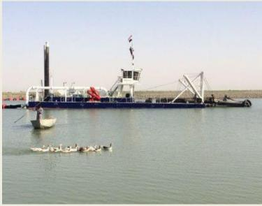
C90 with 350 hp at 2000 rpm. The dredger, fitted with anchor booms and spud carriage, has a crown type cutter with 150 hp and the swing winches have a 6 ton pull. *Equipment:* Arbour gen-set with 30 kW; DGPS positioning system with an integrated project monitoring program; Production measuring system. *(Source: Dredging Today)*
