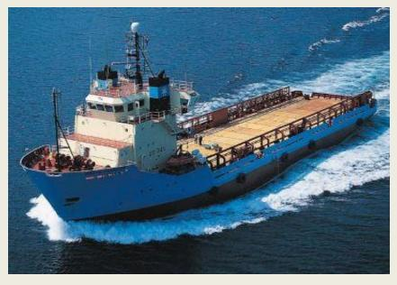
for the PSV that has been hired to support the FPSO, the **Maersk Frontier** is a DP2 vessel which operates in the North Sea. It has a deadweight of 4,600 tonnes and a deck area of 907 square meters. (Source: Offshore Energy Today)
