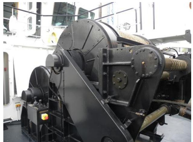
Towing / Anchor handling winch arrangement deck view
