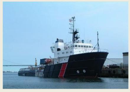
Tunnel, 1 x 500 BHP Tunnel. AH/Towing: Bollard Pull 85 t; Winch Type Single drum tow winch; Winch Pull 140 T; Winch Brake 190 T; Tow wire 1000m x 54mm; Tow Pins 2; Tugger 1 x 5 t; Deck Crane 1.0T @ 6.0m; Max Speed 12.5 knots 1.0 m3/h; Econ Speed 10.0 knots 0.7 m3/h. Standby Rescue Equipment: Rescue Class 280 Survivors; FRC 1 x 15 person; Rescue Basket 1 x Dacon Scoop. Accommodation: Cabins for
