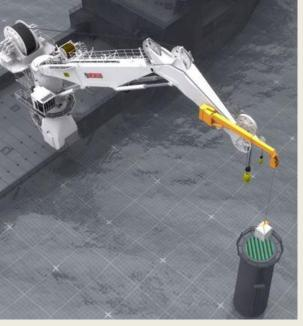
load in relation to a fixed point in space. During operations that require a greater degree of precision than that available from the standard crane, such as transferring equipment to or from offshore wind turbine structures or any fixed platform, the operator can opt to use the 3DMC. "MacGregor recognises that any investment must deliver distinct operational advantages, particularly in today's challenging economic climate," adds Dr Nürnberg. "The 3DMC retrofit option does exactly that. It
