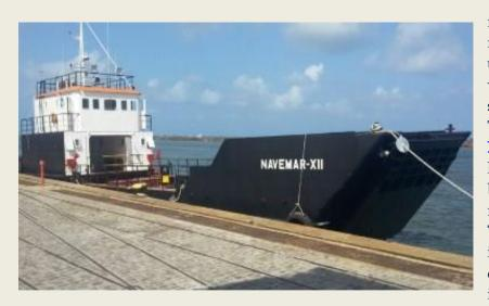
navigating through the region, due to the danger of underwater reefs and strong winds, which might adrift the ship to the rocky shallows. The general cargo vessel Navemar-XII has overall length of 24.00 m, moulded of 4.00 m maximum draft of 2.50 m. The gross tonnage of the ship is 150 GRT. The vessel was operating as coastal freighter in Brazil and during the
