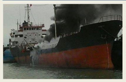
One dockworker died after explosion and fire on board of product tanker Istana V at the dock in Batu Ampar, Indonesia. The vessel was under repairs at the port, but during welding works on the cargo decks suffered explosion of oil fumes. Another two people heavily injured and were transported to the hospital in critical condition. The accident was reported to local authorities and was requested
