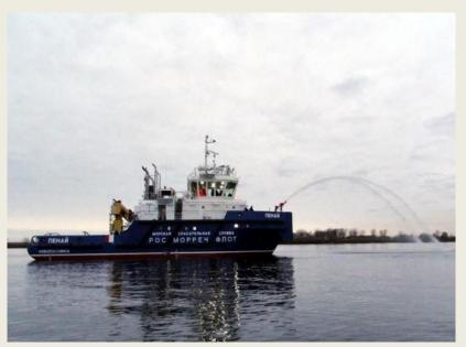
ship designer. The vessel is intended for towing of vessels and floating facilities in marine conditions; participation in oil spill response operations as an auxiliary transport for delivery of dedicated equipment and for installation of booms; assistance in firefighting operations at floating and coastal facilities for transportation of general cargo the deck loading/unloading of cargo by port facilities or onboard crane. The vessel's area of navigation – sea districts corresponding to
