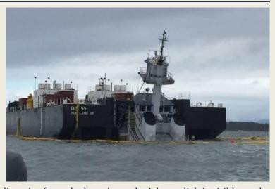
submerged, suspended by its ATB coupling pins from the barge's notch. A large slick is visible on the
