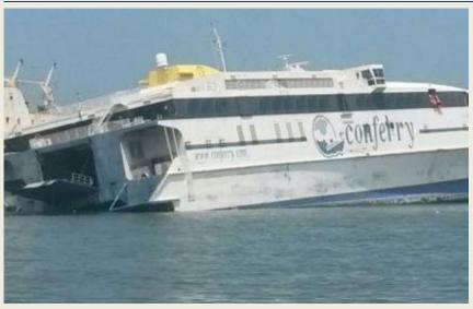
The catamaran ferry Carmen **Ernestina** partially sank at pier in Puerto la Cruz, Venezuela. The vessel suffered breaches in the hull and the port side flooded, the bottom resting leaning the pier, submerged. The ferry was docked at the port since 2 months without maintenance and abandoned by crew. She was under monitoring of the local
