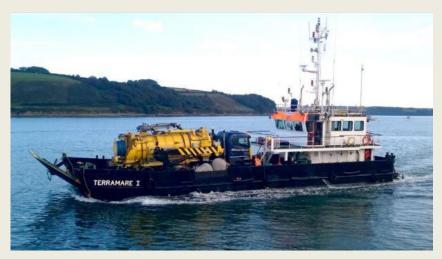
**Terramare** is well suited for offshore dive operations. For station keeping in shallow waters, the MTS Terramare is equipped with two spud legs allowing the vessel to support survey, construction and installation risk management activities. With a draught of 1.4m and a cargo deck measuring 13.7m x 4.6m, the MTS Terramare can transport up to 50 tons
