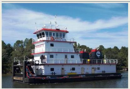
In October, Marquette Transportation Co. took delivery of a new 2,000-hp Z-drive towboat from Master Marine, Inc., Bayou La Batre, Alabama. The 78'x 34'x11' **St. Simon** was designed by Entech Designs, La. For Marquette's river division, based in Paducah, KY. Master Marine is continuing to build "Z-DRIVE" towboats, with one more underway for Marquette with an increased crew capacity of 9 in 5 staterooms with 3 ½
