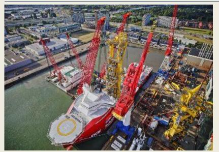
Huisman, the specialist in lifting, drilling, and subsea solutions, welcomed the pipe lay support vessel (PLSV) 'Skandi Buzios' at the its Schiedam quayside for the installation of a 650mt pipelay tower. Scaldis' heavy lift vessel, Rambiz, has earlier this week installed the pipelay tower onboard the PLSV. Huisman said the vessel will be fully commissioned in the next months before it leaves its Schiedam quayside for its first
