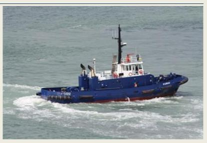
of 4.12 mtrs. The two Niigata diesel engines develops a total output of 2,206 kW (3,000 bhp) (*Photo: Alana Calvert*)
