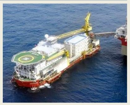
the scope. **Jascon 30** is equipped with a 270 mT heave compensated main crane. The vessel features accommodation for 296 persons, a heave compensated gangway and 700 m2 of unobstructed deck space. The accommodation capacity of **Jascon 30** will be increased with a Portable Accommodation Block (PAB), which will be installed on the deck. Offshore activities are scheduled to commence in October 2016 for a duration of three months firm, with options to extend. *(Source: MarineLink)*
