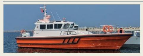
Saqr Port has taken delivery of a new pilot vessel. **Eagle** is constructed from Glass Reinforced Plastic (GRP) and is 15m long, with a beam of 5.1m and working draught of 1.2m. The Eagle,
