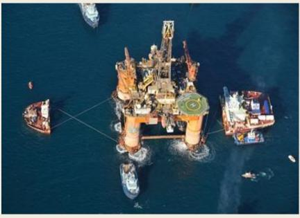
An attempt was made to float the "Transocean Winner" on to the submerged deck "Hawk" on Oct 6. The semisubmersible ship is due to leave on Oct 10 for another job. Work began earlier to submerge the massive deck of the "Hawk" and begin moving the "Transocean Winner" towards the ship. Around noon, the submerged part of the "Hawk" could be seen to be under the rig - ready to
