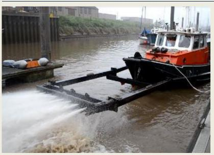
The Marine Group has recently increased their marine service offering with the purchase of a Water Injection Dredger. New vessel is particularly versatile and is capable of dredging in areas out of reach for many larger dredgers. The purchase of the dredger is part of the company's ongoing investment program, which has recently seen the company expand the size of their boatyard. Director of Operations, Freemantle, commented: Water Injection Dredger is a
