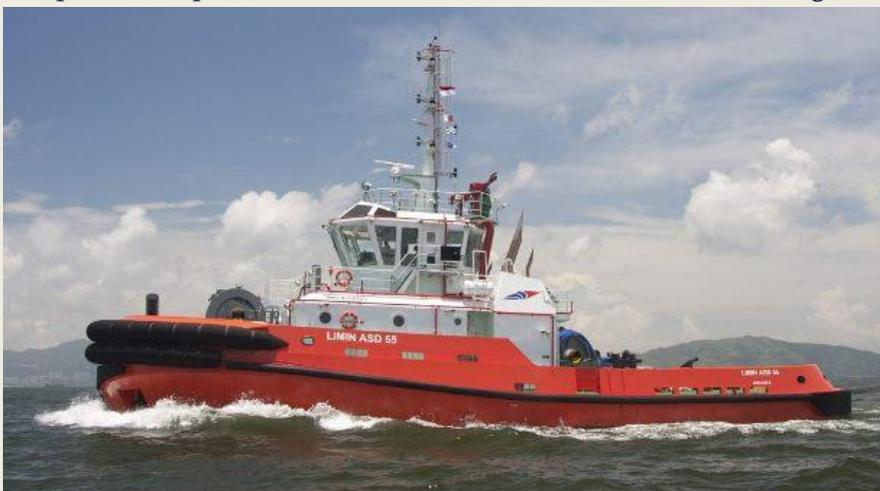
knuckle boom deck crane is installed on aft deck for handling of service parts and small cargo. Main propulsion for each tug comprises a pair of CAT 3516C diesel engines, each rated at 2682 BHP at 1600 rpm, and each driving a Schottel, SPR 1515 fixed pitch Z-drive unit, in ASD configuration. The electrical plant comprises
