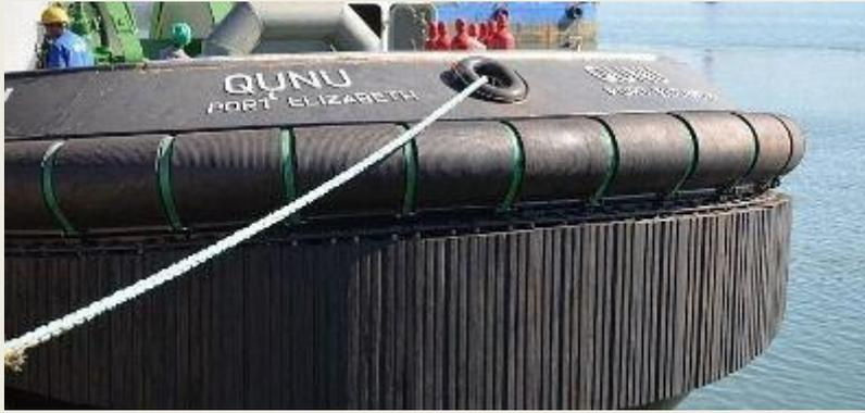
by Southern African Shipyards for South Africa's Transnet National Ports Authority. The scope of supply includes cylindrical, W-type and wing fenders for the new 70 tonnes bollard pull tugs, two of which, **Qunu** and **Cormorant**, were named at the yard in May and entered service in June and July
