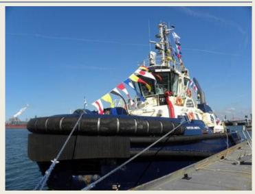
develops a total output of 3,530 kW at 1,800 rpm. driven two Rolls Royce Aquamaster US 205 FP which give the tug a free sailing speed of 12 knots a bollard pull ahead of 60 tons and a bollard pull astern of 56 tons. Her grt is 312 tons, dwt 108 tons and nrt 94 tons. She is classed American Bureau of Shipping with notation ABS+, A1,
