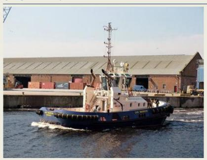
Working away on the Clyde last week berthing a bulker in Glasgow was the Damen built CMS Warrior. The 2015 built tug is a Damen ASD 2310 design with yard number 512916. The Clyde Marine Services tug has a length of 22.71 mtrs a beam of 10.43 mtrs and a depth at sides 4.50 mtrs. The Caterpillar 3512C TA HD+/C main engines develops a total output of 3,000 bkW (4,023 bhp) at 1,600 rpm. Her basic functions are towing mooring operations. She has a
