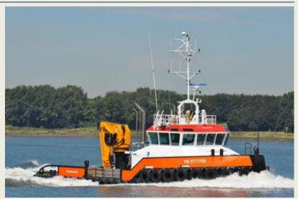
manoeuvrability. Further to her designed for heavy duties with an optimum bollard pull in combination with a shallow draft. The standard Shoulbuster 2709 has a length of 27.19 mtrs a draft of 2.60 mtrs. Her engines develops a total output of 2,238 bkW which results in a free sailing speed of 11 knots and a bollard pull of 38 tons. *(Photo: Ruud Zegwaard)*
