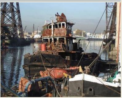
Buenos Aires, beneath the Pueyrredon Bridge. Which is seen on the picture. After 2007 wreck removed by Prefectura Naval Argentina (coast guard). The tug has a length of 32.46 mtrs a beam of 7.02 mtrs and a depth of 3.45 mtrs. The 3 cylinder Wollheim Triple Expansion Engine has an output of 550 ipk. Her brt is 241 tons. Thanks to all who have searching for the details of this tug it is very much appreciated. *(Photo: Historia y Arqueología Marítima)*
