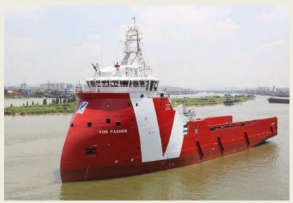
featuring the Ulstein-patented X-BOW design. The PSV complies with ABS class requirements for dynamic-positioning system Class II (DPS-2) and reduced noise and vibration to satisfy a Comfort-Class notation. With a length of 83.4 meters and a beam of 18 meters, the vessel provides 850 m2 of deck space and a load capacity of 4,200 tonnes (dwt). The naming ceremony for the PSV was held in July at the Cosco Guangdong Shipyard, China. *(Source: Offshore Energy Today)*
