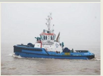
continuous 4000kw power rate of its main engine and 13 knots of its sailing speed, which, ensures itself can be operated in unrestricted area. The class notations of this tug is from ABS, namely ABS Al TOWING VESSEL, ESCORT VESSEL, E, AMS, UNRESTRICTED NAVIGATION, FIRE FIGTHING VESSEL CLASS 1°. The tug is Tuvalu registered with call sign T2WN4 with a grt of 497 tons and a dwt of 298 tons. She is classed American Bureau of Shipping *(Source: Zhenjiang Shipyard)*
