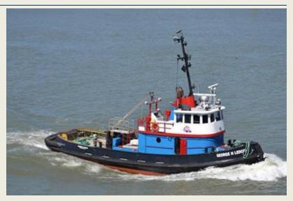
length of 19.29 mtrs a beam of 6.22 mtrs and a depth of 2.99 mtrs. The Caterpillar engine has an output of 700 bhp. (*Photo: Robert Etchell*)
