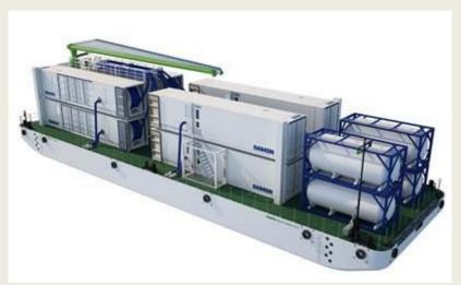
testing onboard the Henrike Schepers. During the shipboard tests, ballast water was taken in untreated and the efficacy of the technology was validated upon discharge. These tests have shown that the InvaSave is capable of providing an IMO type approved backup in a port in the event of a failure in a vessel's on board treatment systems to uptake or discharge ballast water. It can even serve as a port-based alternative for
