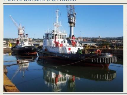
The two tractor tugs, both with Voith Schneider propulsion, are Durban's **Mkhuze** (built 2003 on the left) and Richards Bay's **Uhuva** (ex W Marshall Clarke, built 1974), which have undergone maintenance in the port dry dock. Here the dock has been reflooded prior to the tugs departing for the fitting out quay next to Durban's Shop 24. (Source: Ports & Ships; Photo: Ken Malcolm)
