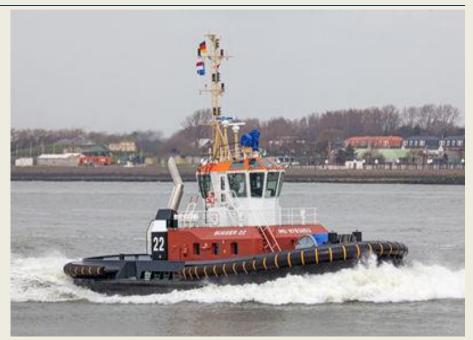
The two Caterpillar 3516C TA HD+/D develops a total output of 4,200 bkW (5,632 bhp). Her bollard pull is 70.1 tons ahead and 67.6 tons astern Her speed is 13.3 knots ahead and 13 knots astern. She has a grt of 268 tons and a dwt of 150 tons. The tug is classed Lloyd's Register X 100 A1 Tug [X] LMC UMS IWS (*Source: Damen*)
