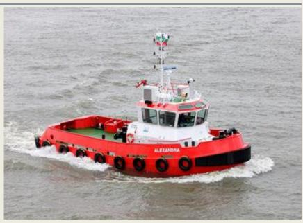
The two Caterpillar C32 TTA Acert / A develops a total output of 1,492 bkW (2,000 bhp). Her bollard pull is 28,5 tons and her speed is 11.7 knots. The tug is classed Bureau Veritas I Hull Mach Tug Coastal Area. (Source: Damen)
