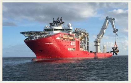
Blue Water Shipping has assisted Sabella and Mojo Maritime in the retrieval of a tidal turbine off Ushant Island in the Celtic Sea. Sabella's D10 tidal turbine was installed at a water depth of 55 m at the site last year, and Mojo Maritime was contracted to retrieve the nacelle in order to check its status. Mojo Maritime used the multipurpose offshore vessel **Aker Wayfarer** to remove the unit from the water. Blue
