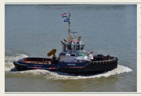
develops a total output of 3,730 bkW (5,000 bhp). Her bollard pull is 62.5 tons ahead and 57.2 astern Her speed is 13.8 knots ahead and 13.6 astern. She has a grt of 293 tons and a nrt of 87 tons. The tug is classed Bureau Veritas I ≝ Hull ● Mach Tug Unrestricted navigation; AUT-UMS (SS) INWATERSURVEY.
