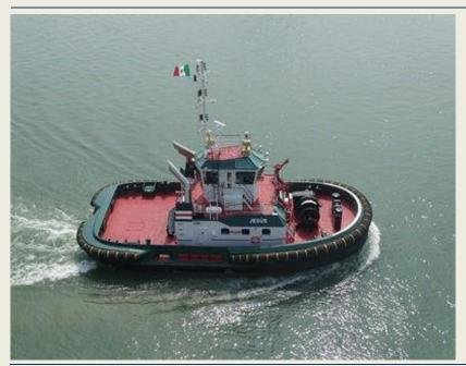
o.a. of 11.33 mtrs and a depth at sides of 4.60 mtrs. Her basic functions are Towing, mooring and firefighting operations. The two Caterpillar 3516C TA HD+/D develops a total output of 4,200 bkW (5,632 bhp). Her bollard pull is 68.8 tons ahead and 65.2 astern Her speed is 13.3 knots ahead and 13.1 astern. She has a grt of 268 tons and a dwt of 150 tons. The tug is classed Lloyd's Register X 100 A1 Tug [X] LMC UMS IWS (Source: Damen)
