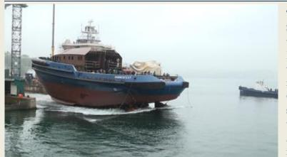
Today, 4<sup>th</sup> July 2016, at Gondan Shipyard in Figueras, at high tide, the first Dual Fuel tug ever built in Europe – and the first of a series of three currently under construction for the Norwegian shipowner Østensjø Rederi – has been successfully launched. Designed by the Canadian company Robert Allan, the new escort tug, with 40.2 meters length and 16 meter beam,
