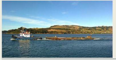
On the 18<sup>th</sup> June 2016 was seen the tug "**Kapu**" in Dunedin upper harbour. She is towing a 32 m split hopper barge. The tug was built in 1983 with a length of 14.46 mtrs a beam of 4.92 mrts and a draft of 2.11 mtrs. The Caterpillar engine develops an output of 520 hp. She has a grt of 55 tons. *(Photo: René van Baalen)*
