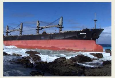
aground in a stable condition with a number of tanks flooded. The deck and side plates of the vessel do not appear to be showing signs of stress. The salvage team managed to relocate within the engine room and preserve and repair in situ one of the starting air compressors of the vessel that had previously been flooded, filled up the air receivers and started of the auxiliary engines, one restoring auxiliary power onboard the ship. The salvage company said that the vessel's cranes and
