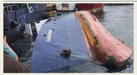
Shrimp trawler **Lavinniy** capsized and sank in Busan port, Korea, in the morning June 21. Korean workers were carrying out repairs the day before, and reportedly, cut off a pipe in engine room, with following water ingress. Vessel capsized and sank, resting by starboard on the bottom, with hull partially above the water.
