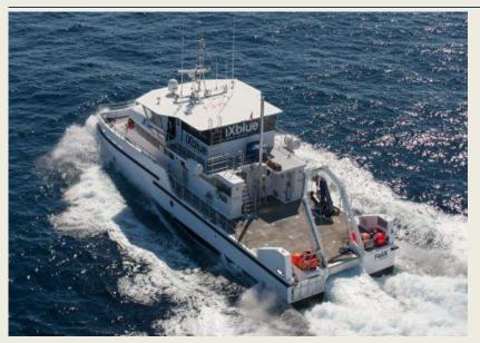
iXblue has baptised its new survey vessel Felix as the latest addition to its iXSurvey fleet. The Felix is a 25-meter catamaran designed to conduct hydrographic, biological and oceanographic missions. The vessel is developed and built by H2X, iXBlue's shipyard in La Ciotat. Built in composite materials, its hull lightweight and non-corrosive. The company markets Felix as complete hydrographic platform, incorporating many
