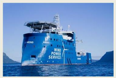
operations, maintenance and servicing of wind turbines. There has been a major focus on the welfare of the technicians who will live on board. While developing the cabins and facilities, the aim has been to position these where the vessel's movements are lowest. The X-BOW, the X-STERN and the integrated DC-based common main drive system, with variable rpm control of the diesel engines for power and propulsion system, are essential design features. In addition to the
