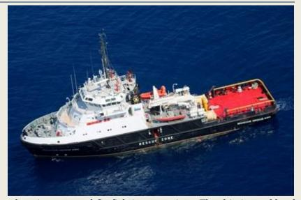
base. The main purpose of the towboat is rescue and firefighting operations. The ship is capable of conducting towing and refloating operations, firefighting and rendering medical assistance, executing difficult diving works at the depths of up to 60 metres. One of its particularities is the
