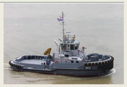
sailing speed is 13.4 knots and the bollard pull 60.2 tons. She has an accommodation for seven (7) persons. *(Photo: Arie Boer)*
