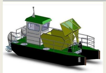
The design team at UK naval Keel architects Marine has developed a compact skimmer vessel that can operate within the tight confines of a small harbour to remove floating debris and weed. With an overall length of 8.10 metres and a draft of just 0.4 metres this skimmer can operate close to beaches and shallow water making it suitable for operation on small inland waterways as well as within the tight confines of a marina. Designed for aluminium
