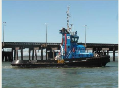
transferred to Smit Lamnalco. She has a length of 32.22 mtrs a beam of 11.24 mtrs and a depth of 5.00 mtrs. The two Caterpillar diesel engines develops a total output of 4,180 kW (5,605 bhp) at 1,600 rpm a free sailing peed of 13.3 knots and a bollard pull of 68 tons ahead and 64 ton astern. *(Photo: Laurens de Bruijn)*
