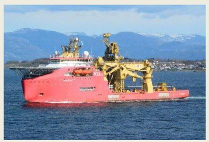
Normand Vison sailing from Rosenberg Verft Stavanger heading for the Gina Grog oilfield west of Stavanger. The Normand Vision is a OSCV 06L design with a length of 156.70 mtrs and a summer draft of 8.50 mtrs. Class definition: 1A1 SPS BIS Clean(Design) COMF(C-3,V-3)Crane(N) DK(+)DYNPOS(AUTRO) E<sub>0</sub> HELDK(H,S) Ice(C) NAUT(AW) Recyclable SF TMON VIBR. built VARD Group AS; Norway.
