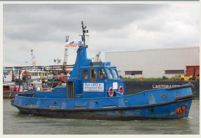
Zonen BV – Sliedrecht and renamed **Leo Jr**. She has a length of of 15.53 mtrs a beam of 5.18 mtrs and a depth of 2.35 mtrs. The Voith Schneider type tug was re-engined in 1972 with a Deutz diesel of 300 bhp. The other tugs in this class are **Lüttje Hörn**, **Mellum**, **Knechtsand**, **Scharhörn**, **Nordstrand**, **Trischen** and **Langeness**. Thanks to the readers for their update information. *(Photo: Leen van der Meijden-2008)*
