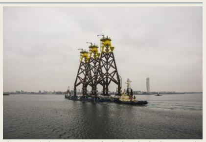
transported to Sassnitz-Mukran, the project's base port located on the island of Rügen. The remaining 29 jackets were constructed in Spain. Blue Water has made an agreement for port
