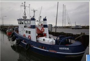
has main dimension 17,22 x 5,50m. GT 52,5, NT 15,7 tons and is fitted with Deutz Diesel 475 BHP and has a Bollard Pull 8-10 tons. Bunker capacity 10.500 ltr and Freshwater 3.00 ltr. Hydraulic Windlass 10 tons and 400 meter and Marinecrane 1 tons. The tug has vent thru a totally upgrade and present itself in a very good working condition. Sole broker in this business has been Bratten Shipping AS, Bergen, Norway. (*Press Release*)
