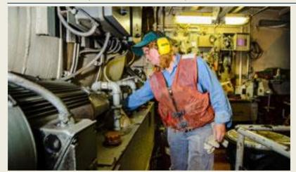
Nancy J.'s power is generated by two EMD 16-TI-149 turbo mains with Twin Disc 540 gears at a 6:1 ratio. At 3,500 hp, Nancy J. is by far the most powerful tugboat in the harbor. The maneuverability, a real feature in a port with no ASD tugs, is provided by four rudders, two of them flanking. "Her power and maneuverability allow us to push sideways on a ship," said
