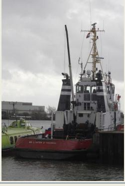
outfitted at Scheepswerf Damen BV – Gorinchem under respectively yard numbers 773 and 8642. In 1987 delivered to Wagenborg as the second under this name Waterman. She has a length of 28.48 mtrs a beam of 9.15 mtrs and a depth of 4.27 mtrs. The two MWM TBD440 mainengines develops a total output of 1,801 kW (2,448 apk). She has a free sailing speed of 12 knots and a bollard pull of 32.2 tons. The tug is classed Lloyd Register of Shipping. (Source & Photo: Jasiu van Haarlem)
