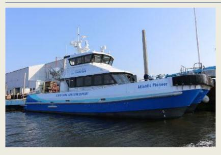
Atlantic Pioneer, the first USbuilt offshore wind service vessel, will be delivered next after recently undergoing sea trials in gale force winds, according to Rhode Island Fast Ferry. The 21-meter crew transfer vessel was built by the Rhode Islandbased Blount Boats to service a 20-year crew transfer contract with Deepwater Wind for its 30MW Block Island offshore wind farm. Atlantic Wind Transfers, Rhode Island Fast
