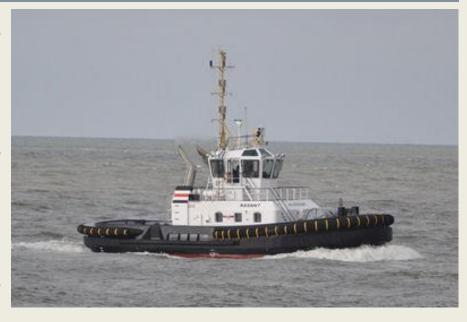
bollardpul of 70 tonnes and a free sailing speed of 13 knots. (Source & Photo: Rob Hoek)
