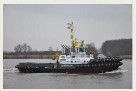
14.3 knots and a bollard pull of 80 tons. (Source & Photo: R&F van der Hoek-Lekko)
