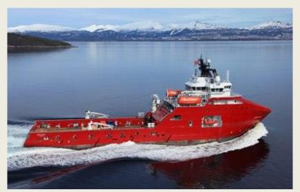
2010-built vessel was designed for deepwater anchor handling during demanding environmental conditions. Skandi Vega is 109m long and operating capabilities include a working moonpool, "Safe Deck" manipulator crane system, a anchor recovery frame, a main winch capacity of 500 T and secondary of 170 T and a bollard pull of 350 T. The vessel has also integrated **ODIM** Anchor
