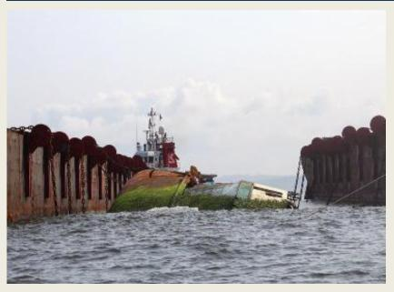
The wreck of a RORO cargo vessel Saloos, which sank at Cabinda anchorage in Angola in May 2014, has been removed from the area by Koole Mammoet Salvage, a wreck removal and salvage company. As the Panamaflagged vessel grounded, its cargo of 155 containers was scattered in an area of 60 km<sup>2</sup> while several containers were stranded on the beach. Koole was hired in 2015 to remove the 4,403 dwt vessel, survey the area, and remove all
