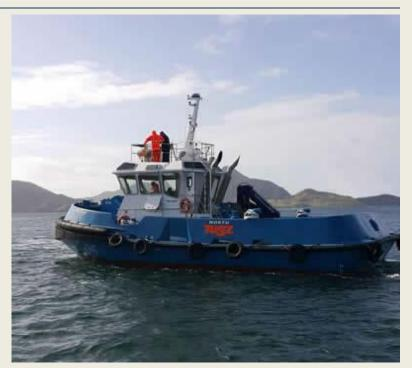
Deck machinery comprises a forward towing winch with 30 tonne capacity, a 30 tonne aft tow hook, 2 tonne tugger winch, deck crane with a 2.65 tonne capacity at 7.9m, a Hydraulic Windlass
