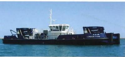
vessel also has a low air draft to allow navigation under bridges upriver as far as Richmond. (*Press Release MacDuff Ship Design*)
