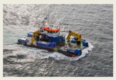
giving a 20m corridor. This work is done in order to clear the route prior to the installation of the export cable. The **Anna-B** will arrive on location at or around 9 February 2016. The vessel will be working in the area for an expected duration of maximum 28 days. (Source: Offshore Wind)
