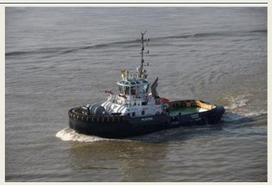
bhp). Her bollard pull is 61 tons ahead and 56.9 astern Her speed is 13.9 knots ahead and 13.6 astern. The tug is classed Bureau Veritas I Hull Mach Escort tug-Fire fighting ship 1 -water spraying Unrestricted navigation. (Source: Damen)
