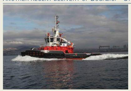
BOGAZICI was awarded the Tender of "Rescue Services of Seaports Szczecin Swinoujscie SA" of POLAND for new building FiFi1 tug boat with propulsion system. special FiFi1 tug boat is fully equipped for safe operations at LNG environments and FiFi services at port, with additional diesel driven fifi pump of capacity 1200 m<sup>3</sup>/h and special Storz coupling sets. Main Particulars of "BOGAZICI 21"
