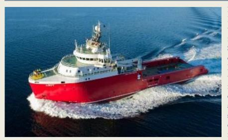
Norwegian shipbuilder Havyard Ship Technology will name its newest icebreaker Aleut at Skoltekaien quay in Bergen on Saturday. Featuring a length of 86 meters and a width of 19,5 meters, Aleut is designed and built to operate under extreme arctic conditions. Havvard said that the icebreaker class ship can break onemetre-thick ice at 3 knots,
