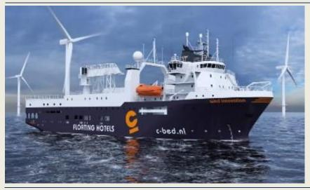
Dutch ship owner C-Bed has contracted Wärtsilä Ship Design to supply the design for rebuilding its seismic survey vessel, the Viking II, for use as a hotel vessel to accommodate and transfer service personnel working on offshore wind farms. After the conversion, the vessel will have accommodation and hotel facilities for 125 people and
