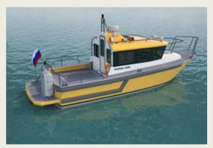
aluminium patrol boat for use by port control authorities and traffic inspectors. The boat has an overall length of 10.3 metres and a beam of 3.41 metres. The boat is equipped with a Volvo D9-430 engine with 32kW and can travel at speeds of 32 knots. The structure of the craft is in aluminium alloy, and the craft two features watertight bullheads. The forward cabin features two bunks, a table and a steering settees, station, toilet. Eight pantry and
