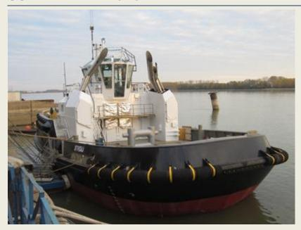
Last week the Damen ASD 2913 with yard number 513103 tug SST Rambala (Imo 9773882) for SAAM SMIT Towage, was launched at the Damen Galati Shipyard - Romania. The ASD 2913 standard tug has a length of 28.90 mtrs a beam of 13.23 mtrs. Her total engine output is 5.050 bkW and results in a free sailing speed of 13.7 knots and a bollard pull of 80 tonnes. This vessel has excellent seakeeping superb behaviour, manoeuvrability and outstanding towing
