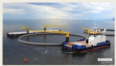
Frøy Vest AS from Norway, for delivery of a *Stan Pontoon 4113* (YN 523702) and a **Multi Cat 2712** (YN 571725). The event took place at Damen Shipyards Hardinxveld, the Netherlands. The Multi Cat 2712, with a length of 27.27 metres, a beam of 12.50 metres and a maximum bollard pull of 34.8 tonnes, is a new type of workboat featuring considerable innovation. The vessel
