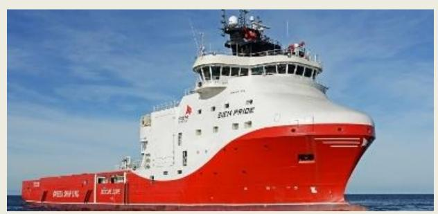
the Polish yard and is contracted for work on a Shell field in the North Sea. **Siem Pride** is 89m long with a beam of 19m and deadweight of 5,500 tonnes. It has an active heave-compensated crane, is fitted for remotely operated vehicles, firefighting, oil spill recovery and rescue and standby services for up to 300 persons. It also has a Safe Hose Operation System and is a class DP2 dynamically positioned vessel with gas-electric propulsion. (Source: Offshore Support Journal)
