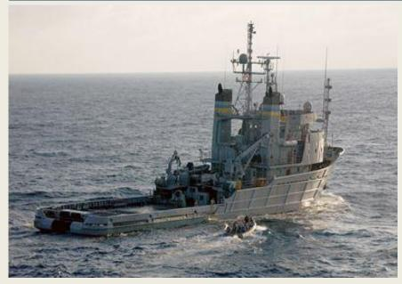
The U.S. Navy is outfitting its towing and salvage vessel USNS Apache with remotely operated vehicles to search for the wreck of the El Faro, believed to be on the bottom in 15,000' of water northeast of Crooked Island in the Bahamas. The 226'x42'x15' 7.200 hp Powhatan-class fleet tug is undertaking the search under contract with the National Transportation Safety Board, which is leading the investigation
