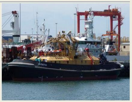
maintenance saving. Compact and powerful, these ATD Tugs have a bollard pull of 43 tonnes, a length of 29 metres, a beam of 9.98 metres, a maximum speed of 13.2 knots and a propulsion system of two Caterpillar 3512C HD engines with a total power of 3,000 bkW at 1,600 rpm. They are also outfitted with Rolls Royce US 205 azimuth thrusters. *(Photo: Aad Noorland)*
