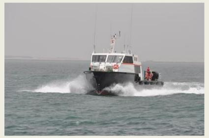
On the 9th September 2015, Grandweld Shipyards accomplished а significant milestone by signing a contract with International Naval Works to design, build and deliver three 21.3 M Aluminium Crew Boats. The 21.3 M vessels will be powered by 2 high speed marine diesel engines; each driving fixed pitch propellers through a reverse-reduction gearbox to produce a speed in excess of 21knots.. The vessels
