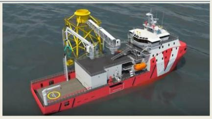
for offshore-access system. They are equipped with two fuel-efficient, super-silent tunnel thrusters and one retractable bow thruster. The vessels will be fitted with 24/7 Broadband communication, Ku-band satellite services with high-performance connectivity with multi-megabit speeds, internet, voice & video streaming with real-time connectivity at sea. Both vessels are currently under construction and due for delivery to Vroon in 2016. Watch the video click HERE (Source: Vroon)
