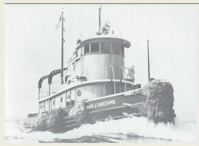
Pushing a huge bow wave, the diesel tug Marie J. Turecamo heads for an assignment under full power. She carries truly impressive rope fenders, and her steel superstructure with painted-on wood grain indicates that owners care about appearance. Built in 1952 Jakobson Shipyard of Oyster Bay, New York under number 340 for Turecamo Maritime. The tug was later acquired by the R.J.Casho Marine company where she was renamed as the Marie J. She was
