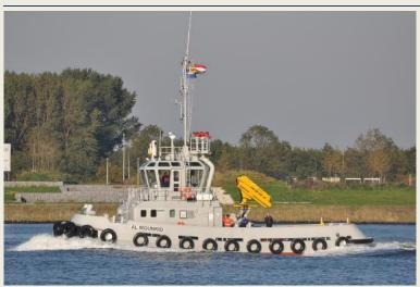
Today, 12th October 2015, late afternoon the maybe last Damen Stan Tug 2208 completed in Gorinchem came to Europoort for technical trials, speed and bollard pull test. Named Al Mounkid, most likely when completed she will show the "name" A02 and will be based in Casablanca.. The standard Stan tug 2208 tugs has a length of 22.60 mtrs and a beam of 7.8 mtrs. Her engine output is 2,029 bkW with a free sailing speed of 12.1
