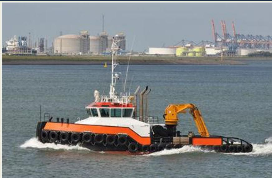
free sailing speed of 11 knots and a bollard pull of 38 tons. *(Photo: R&F van der Hoek-LEKKO)*
