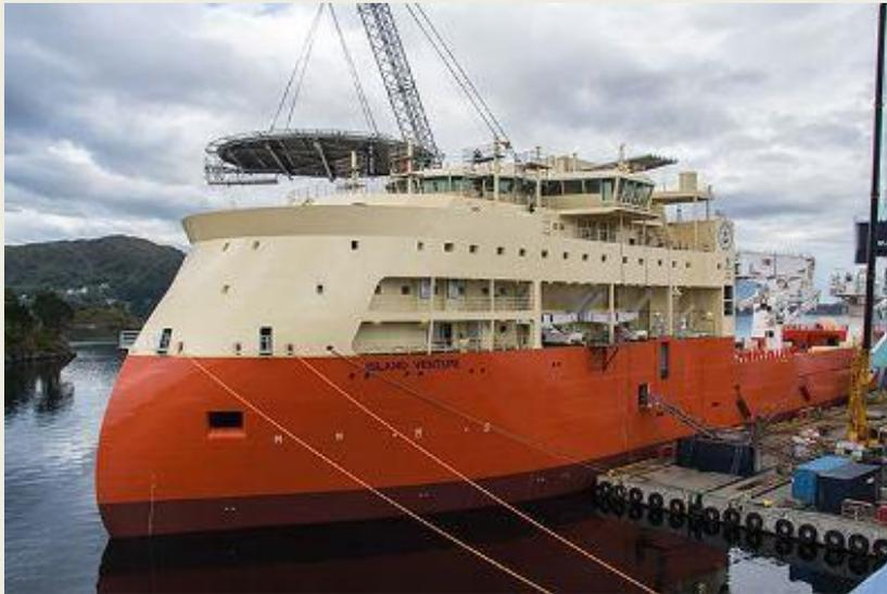
On Tuesday night, yard number 302, **Island Venture**, an offshore construction vessel for Island Offshore/Edison Chouest Offshore, was launched from the dock hall at Ulstein Verft. Currently, the heli deck is being mounted. Measuring close to 160 m in length, and with a beam of 30 m, she is the largest offshore vessel so far from Ulstein Verft. The vessel is jointly owned by Norway-based Island Offshore and US-
