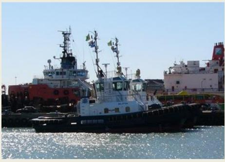
grt of 270 tons and a dwt of 150 tons. The total engine output is 4,200 bkW wit a speed of 13 knots and a bollard pull of 70 tons. *(Photo: Aad Noorland)*
