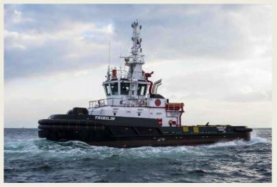
tugs are Cintranaval - Defcar -Spain design type CND32.5/70. They have a length of 32.50 mtrs a beam of 11.70 mtrs and a design 4.30 mtrs. The Caterpillar type 3516C develops total output of 4,200 kW (5,632 bhp) at 1,600 rpm. They have a free sailing speed of 12.5 knots and a bollard pull at 100% MCR of 70 tonnes. Interest can contact David H. Gavan & Sons Shipping gavan@gavan.eu (Source: David H.Gavan)
