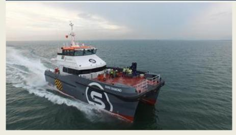
Surewind Marine's, Sure Diamond the first of 2 StratCAT 26m vessels built by Strategic Marine, designed by BMT Nigel Gee. successfully completed sea trails over the weekend. Sure Wind Marine run a fleet of windfarm service vessels (CTV, PSV, Dive vessels and survey vessels) to meet the needs
