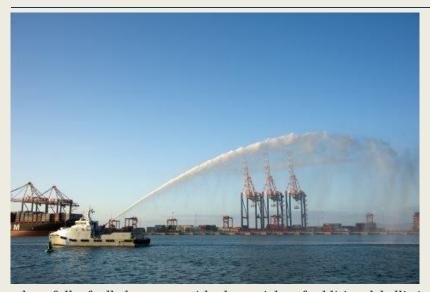
Featuring significant upgrades to meet the vessel owner's requirements, Nautic Africa, a Paramount Group company, launched two new bespoke 35m Sentinel vessels in Table Bay Harbour last week. The vessels were custom designed and manufactured for a Nigerian logistics provider. Nautic's latest builds, AUGUSTINA II and PRINCESS EBIKENIE, are capable of top speeds of 29 knots, and can reach 26 knots
